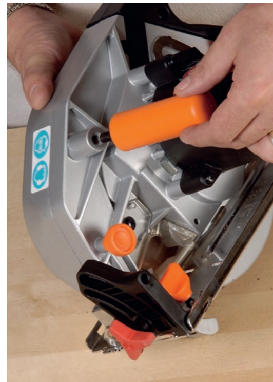
▲ The front handle can be moved back to a middle position if necessary
