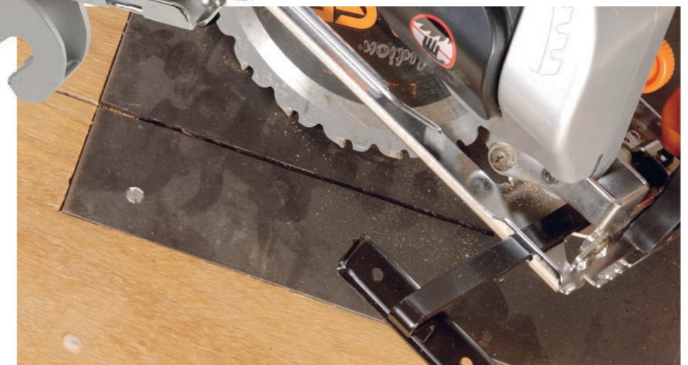
▲ This steel plate is 4mm thick and the ply is 19mm. The saw didn't flinch!
